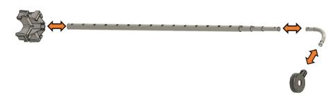
Insert Tubes into the Tube holder, the Bend Piece and Detector Holder.
